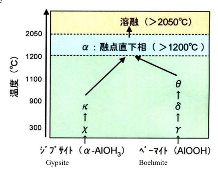
Figure Phase transition of aluminum oxide (Al<sub>2</sub>O<sub>3</sub>)
